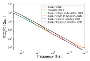
Figure 4: Transverse dipolar impedance (real part) versus frequency for a 10 km long chamber, with inner radius r = 20 mm.
