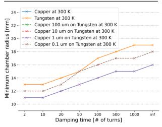
Figure 5: Minimum chamber radius required to keep the emittance growth below 10 % after 3000 turns, for the different copper coating thickness considered and pure copper or pure tungsten (no copper coating).
