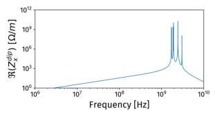
Figure 2: Transverse dipolar impedance (real part) versus frequency. 696 cavities are assumed in the model, and all transverse HOMs from the Low-Loss TESLA type cavity are included.
