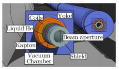
Figure 3: Radial scheme proposal for the collider magnets. The shield's function is to intercept muon decay products and protect the superconducting coils. Picture courtesy D. Calzolari [15].
