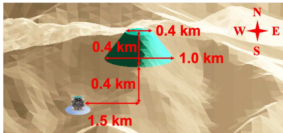
Figure 8. The mountain (grey) with an artificially embedded density variation region (cyan) and its shape and location. The height and diameter of the detector are enlarged 100 times for display convenience. The horizontal distance from the detector to the center of the region is 1.5 km.
