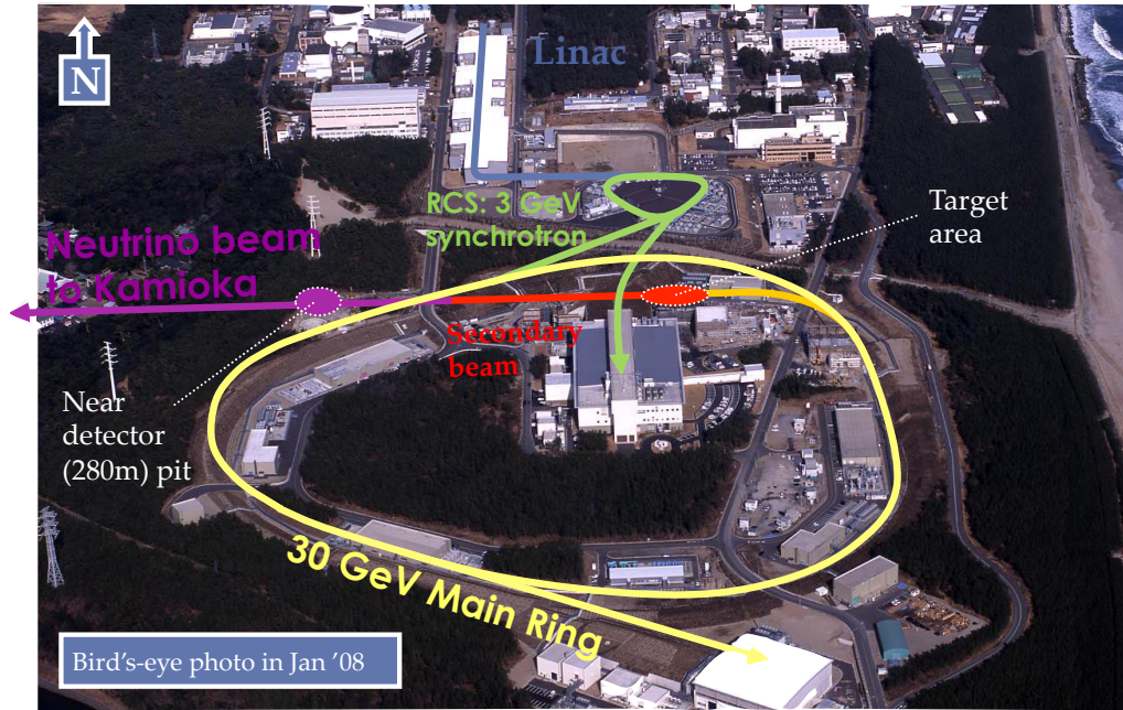
FIGURE 4.3: Photo of the J-PARC accelerator with diagrams overlaid. The proton beam starts in the LINAC and then is accelerated first to 3 GeV in the RCS then to 30 GeV in the main ring. The protons are then extracted from the main ring into the secondary beam line where they are directed into a graphite target. Particles produced by the interaction of the protons and target eventually decay into the neutrino beam directed along the path shown. Figure from the J-PARC website.
