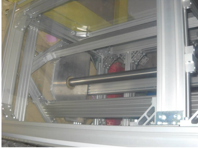
FIGURE 4.5: Photo of the target assembly protruding from the center of the first magnetic focusing horn. Photo by K. Mahn.
