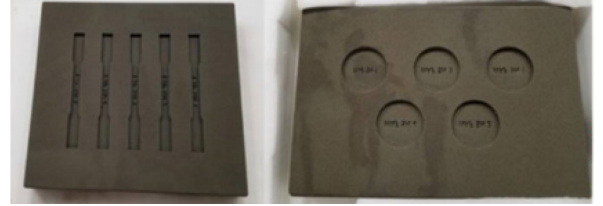
Fig 1: Bottom half of 3D printed sand molds
