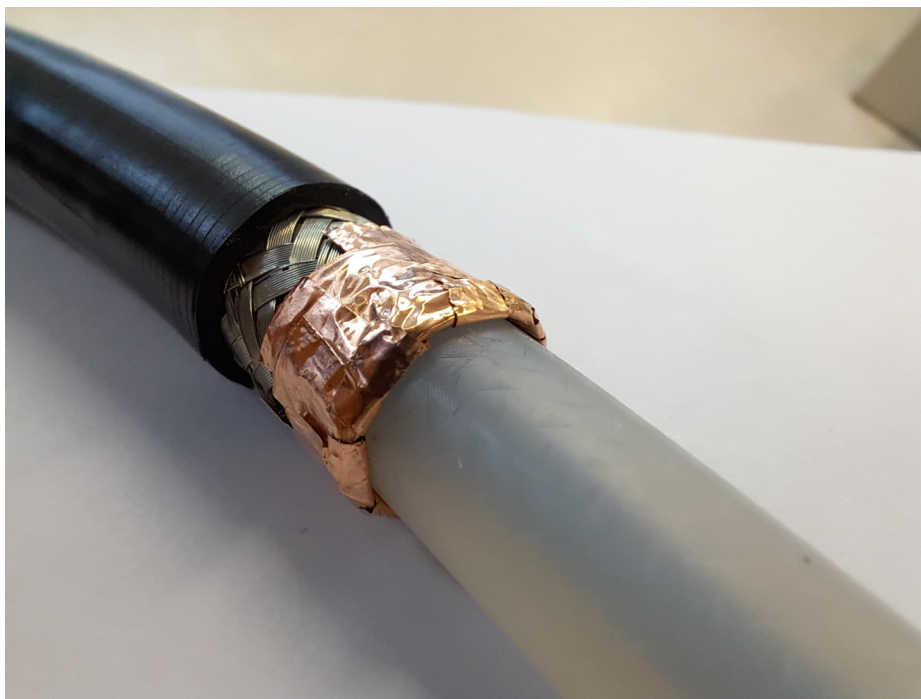
Figure 2.25.: The grounded mesh is removed on the load side, and special care is taken to cover the pointy ends of the grounded mesh with conductive (copper) tape.
