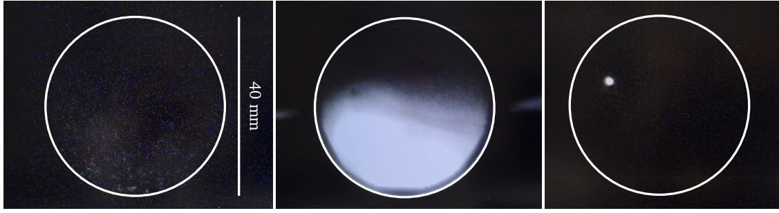
Figure 3.17.: Images of the MCP with no magnetic field (left), <0.15 T (middle) and >0.15 T (right). The increase in intensity is the effect of the magnetic field guiding the electrons along the field lines. The white circle indicates the extent of the 40 mm phosphor screen.
