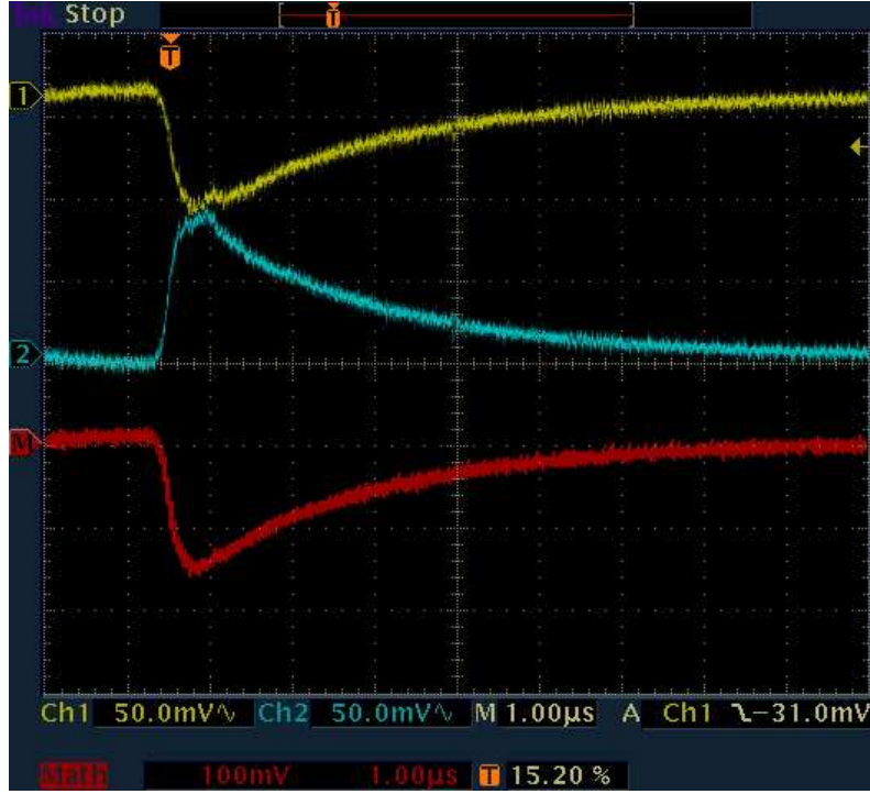
Figure 3.8: Analogue signal from a cosmic muon event recorded with an oscilloscope at the output of one preamplifier channel [43]. The negative (1) and the positive (2) outputs are shown as well as the difference (M).
