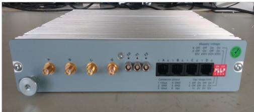
Figure 3.20: Picture of the data acquisition electronics module.
