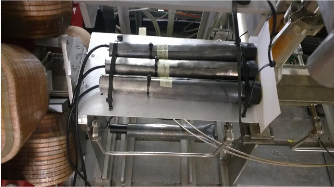
Figure 3.13: The lead shielded detectors installed in the storage ring.
