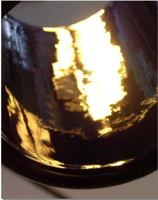
Figure 1: Glasslined technical equipment with extremely smooth surface finish in conjunction with high wear resistance to abrasive acting media and high resistance to corrosion.
