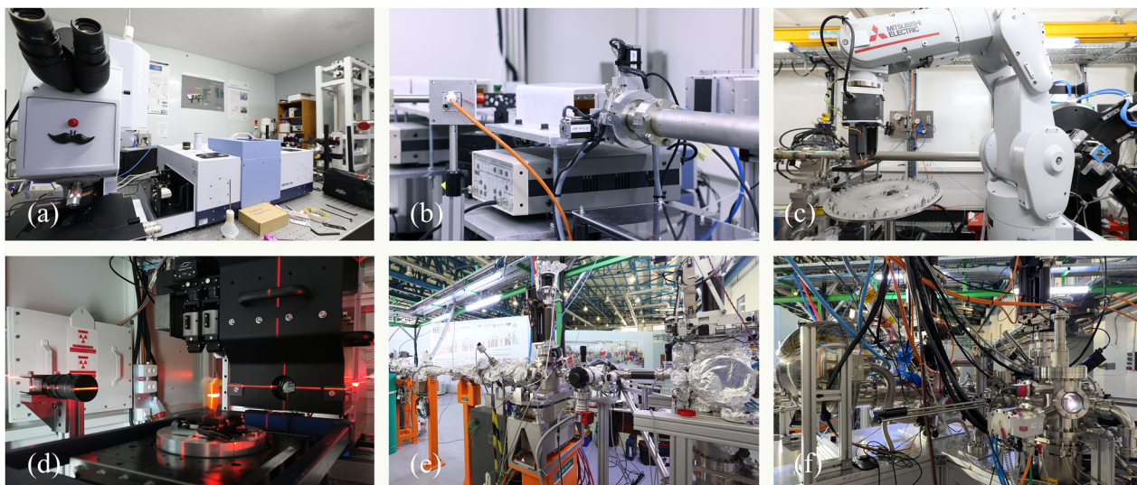
Figure 3. Experimental setups at SESAME. (a) The IR microscope and the spectrometer at the BM02-IR beam-line; (b) the ionization chambers and the AXPiDe at the BM08-XAFS/XRF beam-line; (c) the sample changer and the powder diffractometer at the ID09-MS/XPD beam-line; (d) the sample stage and the detection setup at the ID10-BEATS beam-line; (e) the last focusing mirror and experimental chamber at the ID11L-HESEB beam-line; (f) the experimental station at the ID11R-TXPES beam-line—TXPES beam transportation components are expected in SESAME in spring 2025. (Photo credits: a, b, c, e: Giorgio Precali; d, f: SESAME).
