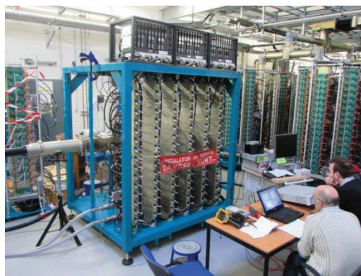
Figure 4: ThomX 50 kW, 500 MHz SSA constructed at SOLEIL and presently under testing.
