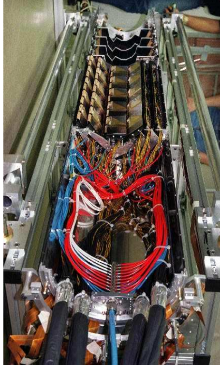
Fig. 40. A photograph of one half of the MVD, showing the barrel ladders, one half of each of the four forward wheels and the cables and services.
