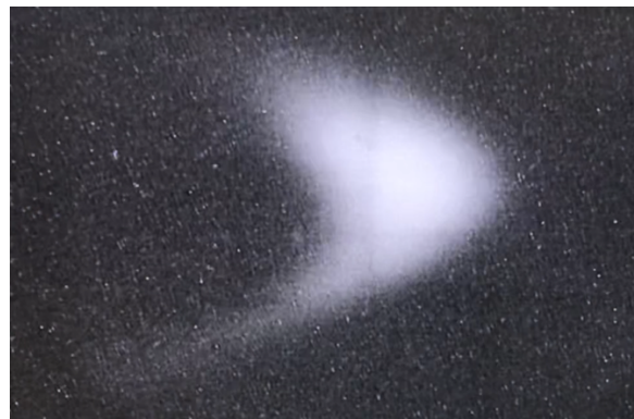
Figure 1: Pre-upgrade beam viewed on a phosphor screen after drifting 9.2 m from the booster extraction septum.
