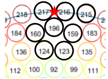
Figure 4.13: Zoom of one area on the top PMT array. The PMTs marked in black are the ones switched off for this study.
