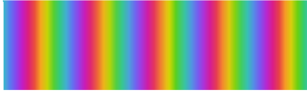
Figure B.1: An abs-arg plot of a plane wave demonstrating its linear phase profile.
