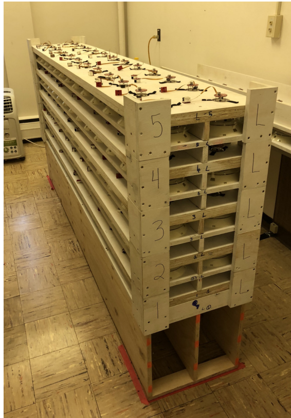
Figure 4.26: The jig for PMT potting. Alternating layers of PMTs and covers were stacked and the tubes were held straight during the curing process.
