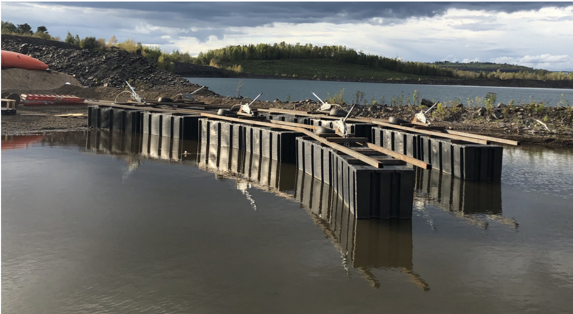
Figure 4.13: Two one-quarter segments of the floating dock. Three winches spaced between six floats were mounted on top.
