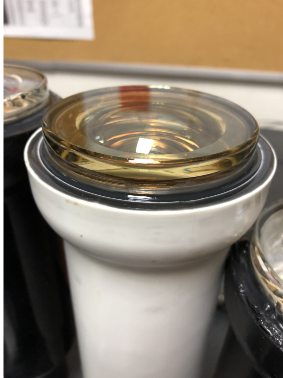
Figure 4.29: The photocathode of a Madison PMT exposed to the environment. The tube was glued into the white insert with black resin that created a waterproof barrier.
