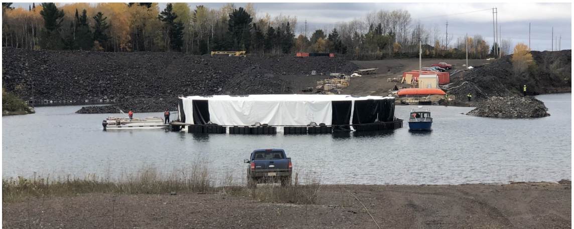
Figure 4.42: The exterior of the detector after completion. The liner can be seen supporting the detector and the floating dock forms a perimeter around the detector. The two boats tow and steer the detector during deployment. The scale of the detector is visible.
