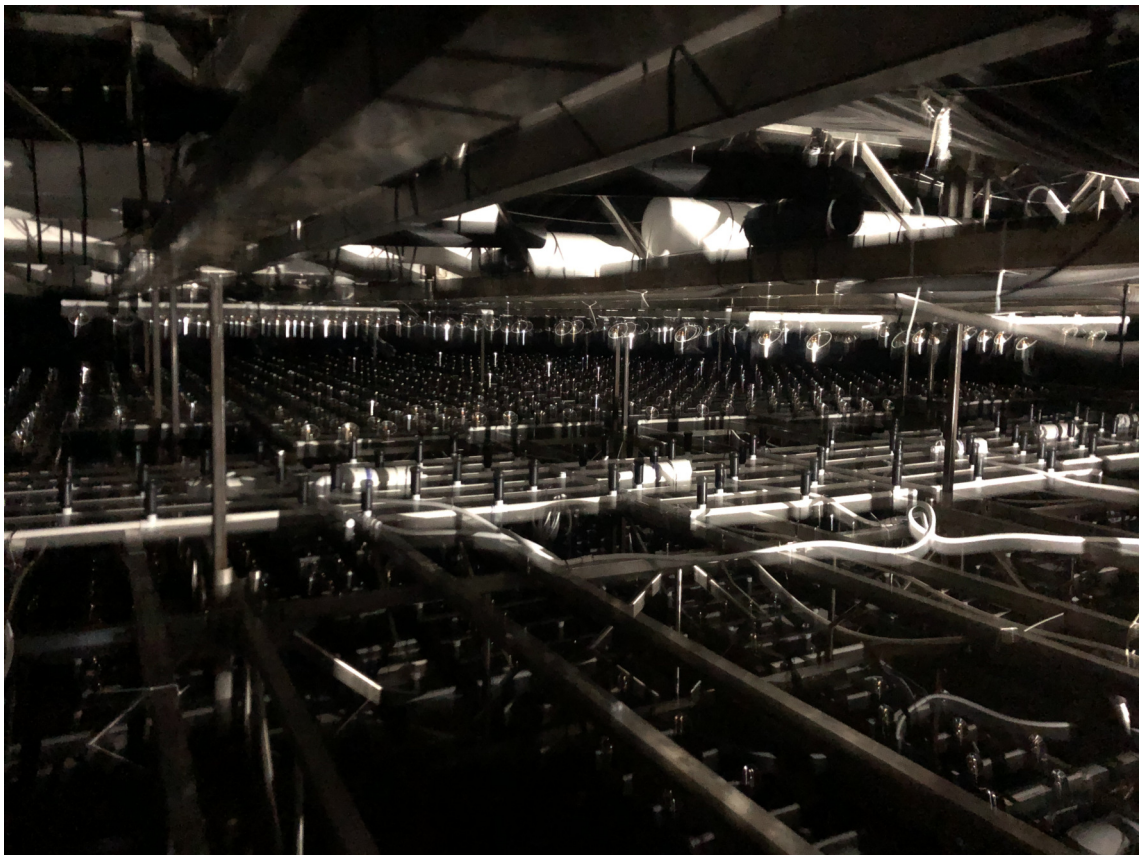
Figure 4.45: The detector from the front during the final liner sealing process so the detector was and waterproof.
