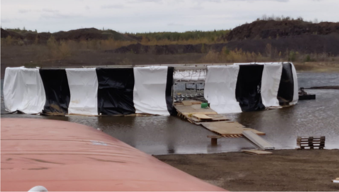
Figure 4.11: The detector completely wrapped in liner. Additional liner was folded around the base below the water line so that the detector could stretch to be 12 m tall.
