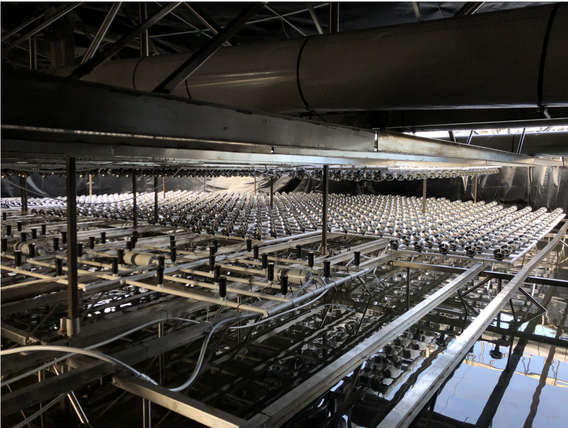
Figure 4.44: The interior of the detector: the rows of Nikhef PMTs angled to point into the neutrino beam can be seen at the back with the Madison planes in front. The top cap buoyancy can be seen above.
