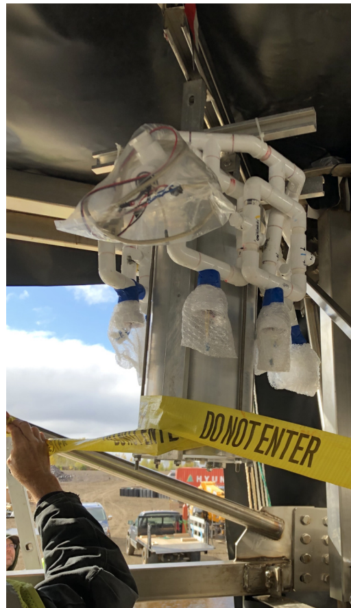
(b) The exterior of the main control box installed inside the detector. The PVC fitting attached to the aluminium container contains resin for preventing any leaks in the manifolds entering the container.
