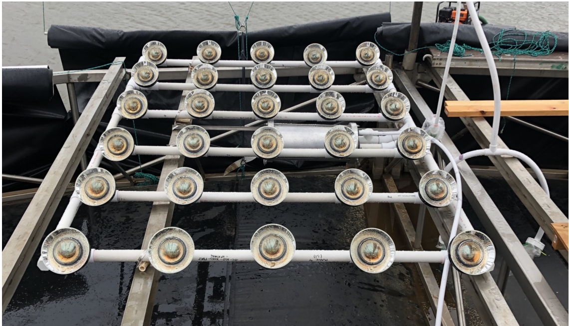
Figure 4.24: A Nikhef plane installed inside the detector. The PMTs were angled forwards into the beam and the aluminium electronics container can be seen in the middle. The PVC hose exiting the electronics container was for connecting the plane to cable manifolds which lead to fanout containers.
