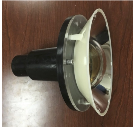
Figure 4.22: The assembled PMT with its plastic reflector attached ready to be glued onto a plane.
