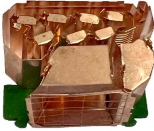
Figure 3.6: The internal dynode structure of a PMT. The first dynode is at the front covered by a copper mesh and the chain of dynodes can be seen behind in an alternating ladder arrangement.
