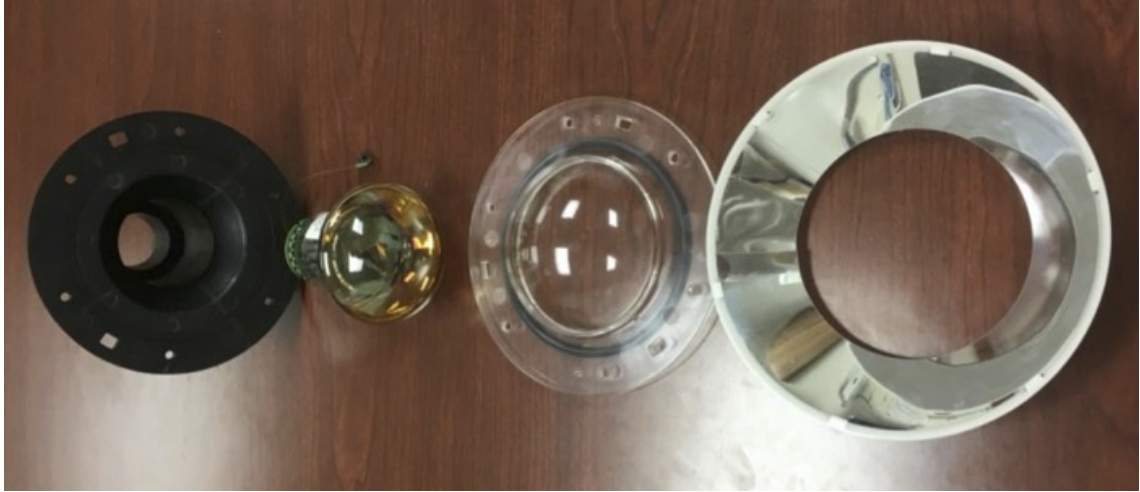
Figure 4.21: A fully disassembled Nikhef PMT showing from left to right: the PMT insert, the PMT itself with its high-voltage base attached, the waterproof cover complete with its O-ring and then the plastic reflector for light.
