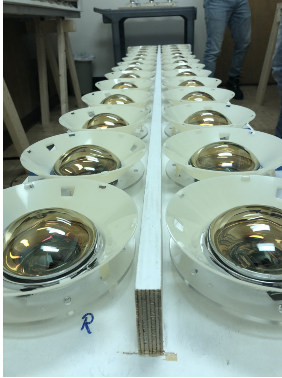
Figure 4.27: A row of PMTs after the potting process showing the consistency of the transparent finish that can be achieved by potting the tubes.
