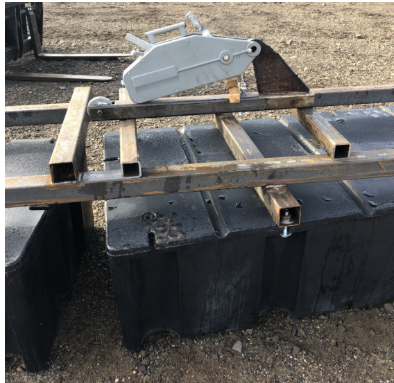
Figure 4.14: One of the winches used in CHIPS mounted onto the floating dock. The 12 winches could lift a total of 19 tonnes of dry mass.
