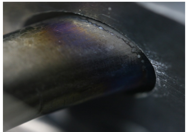
Figure 5: Evidence of possible arcing in the prototype.
