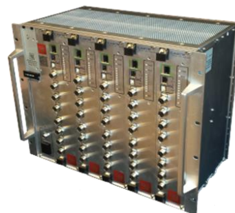
Figure 5. 5 CABTR boards integrated in 19" crate (40 available channels)
