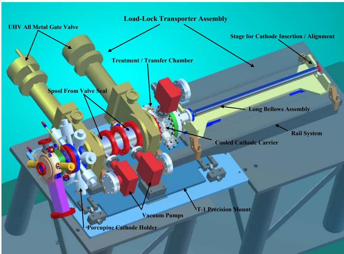
The load lock approach adopted by SLAC requires two load-lock transporters: one mounted on the gun and another in the cathode processing lab where cathodes are prepared and stored for use on the gun. A single cathode is mounted in each transporter, eliminating the need for transferring cathodes under vacuum from a storage carousel, or
