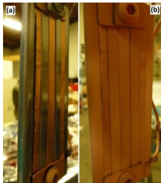
Figure 9: SS 316L strips, (a) before and (b) after 30 \mu\text{m} copper coated film.
