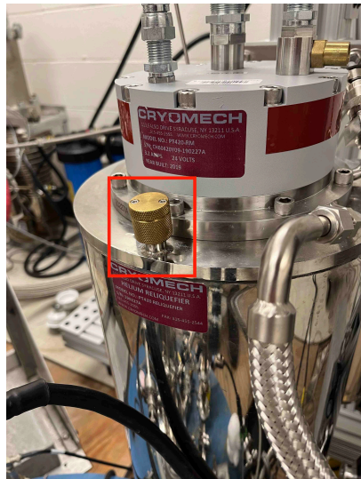
Figure 1.46: The Cryomech cold head can be filled with liquid Helium directly using the fill port shown here.
