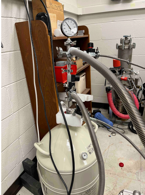
Figure 1.47: Image of the liquid Nitrogen cold trap used in our experiments. The ^3\text{He} insert 1 K pot is pumped using a rough pump and the output can be pumped through the cold trap (the high impedance lower segment is immersed in liquid Nitrogen) to clean the Helium of impurities before recycling it. The flow is directed using the various Speedivalves shown in the picture. The pressure gauge at the top is used to indicate when the cold trap needs to be regenerated.
