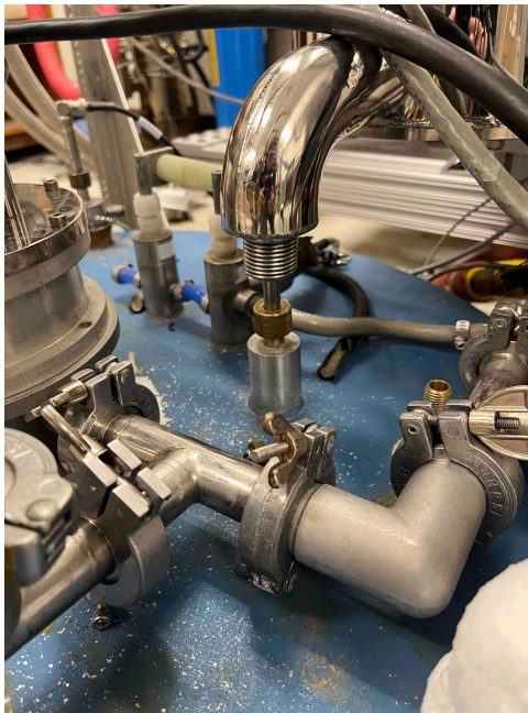
Figure 1.45: The Cryomech transfer tube is inserted directly into the liquid fill port of the 15 T cryostat.
