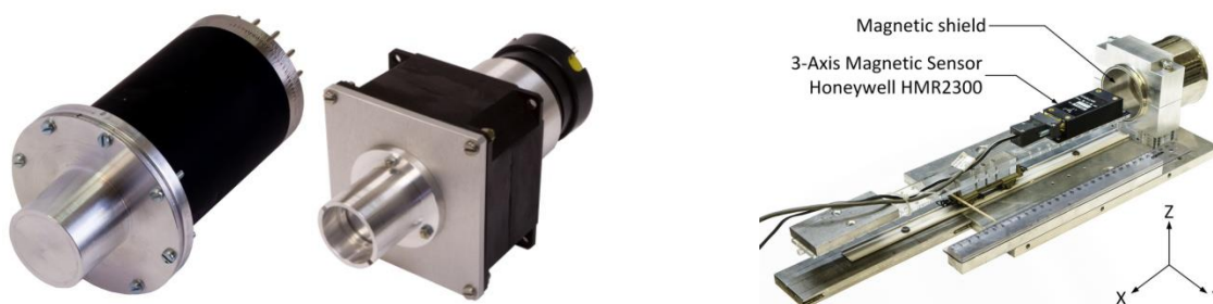
Figure 1. The \text{LaBr}_3(\text{Ce}) crystal with R6231-100 and R6233-100 PMTs detector assembly. Figure 2. HMR2300 magnetometer based setup.
