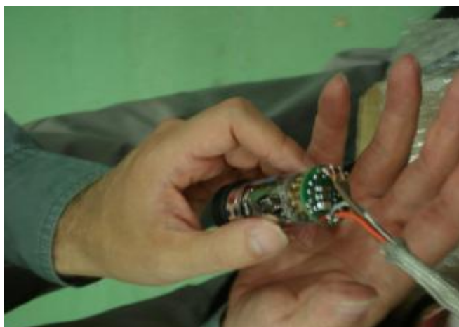
Figure 4.12. CASTOR PMTs on top of the light guides and bases used in the 2007 beam tests
