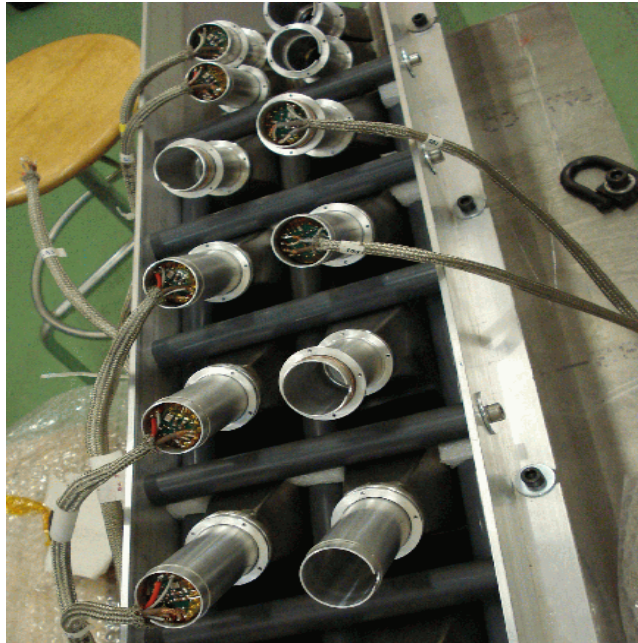
Figure 4.12. CASTOR PMTs on top of the light guides and bases used in the 2007 beam tests
