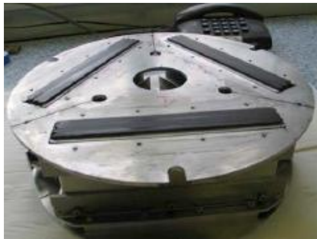
Figure 4.7. Lapping machine (upper), Lapping-polishing tool turned upside down to show the edge of 3 stacks after lapping (bottom)
