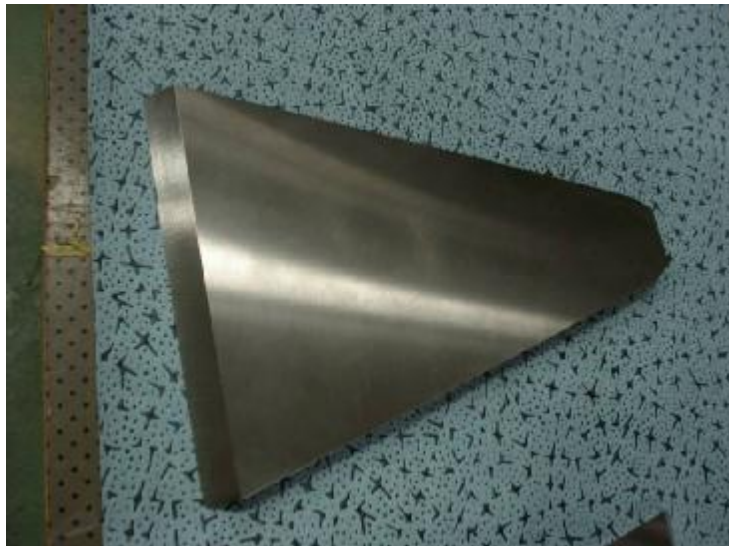
Figure 4.1. Example of a tungsten plate used for the assembly of prototype III.
