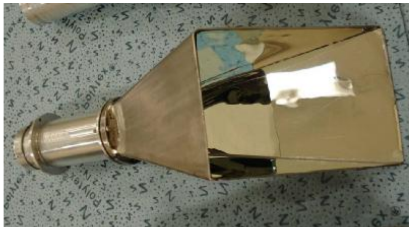
Figure 4.10. Air-core light guide designed for prototype III and reflecting foil covering inside
