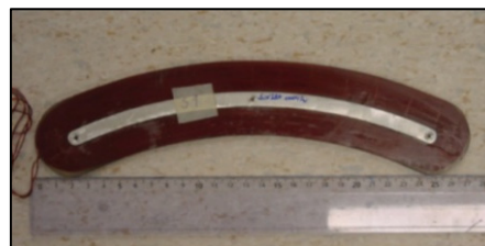
Figure 5: Harmonic coil in the prototype.
