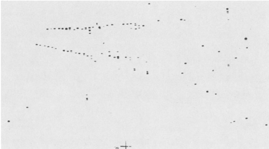
Fig. 4: "Naked" \pi^0 \rightarrow 2\gamma , initiated by hadronic neutral current in the AC-PD sparkchamber.
