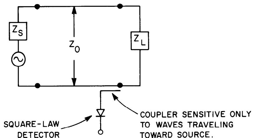
The generator is a voltage source, capable of delivering a constant voltage regardless of load impedance. The coupler is assumed to introduce negligible loss and reflection, and to have infinite directivity. The detector is assumed to be perfectly square-law.
