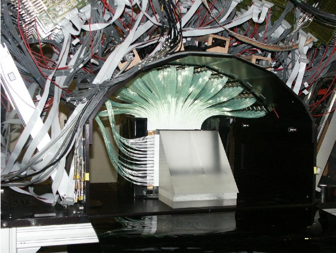
Figure 3.11: The final FAST target, including the wedge, the  $z$ -counter hodoscope and the magnet plates on the two sides of the target.
