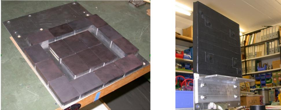
Figure 3.9: Left: An array of (not yet) magnetized ferrite blocks arranged on the aluminum plate support. The outer thick ring provides the main field, the inner thinner blocks improve homogeneity. Right: One of the two ferrite plane assemblies, ready for installation. (Dimensions:  $30 \times 30 \text{ cm}^2$ ).
