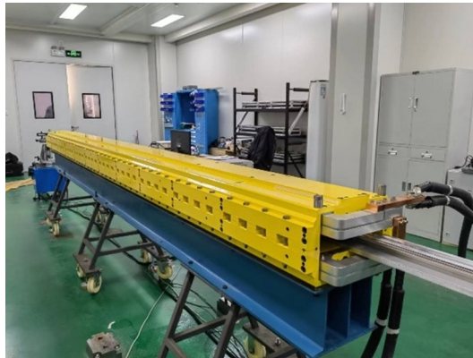
Figure 4. CEPC booster full size dipole magnet.
