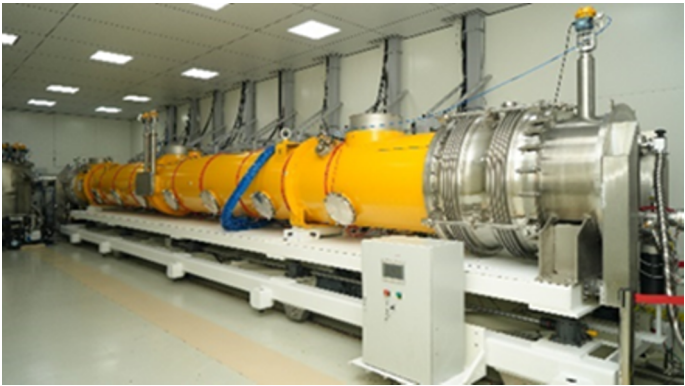
Figure 2. CEPC 1.3GHz full size cryomodule.
