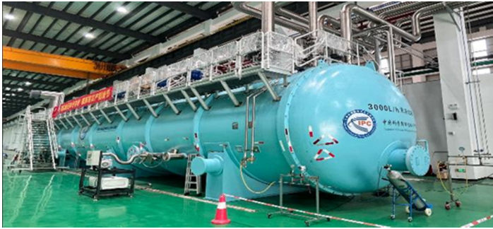
Figure 5. CEPC 18kW@4K cryogenic refrigerator.
