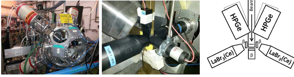
Figure 1. Left and central panels: pictures of the experimental setup. The left panel shows the holding structure of the clover detectors, placed backwards as respect to the beamline, while in the central panel a detailed view of the fast-timing setup is visible: to the sides we see the two LaBr 3 (Ce) detectors, each of them facing a thin plastic detector directly attached to the beamline, while in front of the implantation point another fast-responding plastic detector is placed. A schematics of the detectors' arrangement is presented in the right panel.
