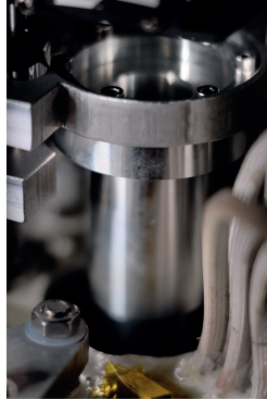
FIGURE 4.7: A close up picture of the tweezer objective mounted inside the MOT coil. The objective must be aligned orthogonal to the window and suspended just above the window (0.9 mm from the front face of the objective to the window) such that the tweezers can be aligned to the red MOT. We had to modify the objective mount assembly in order for it to pass the MOT coils.
