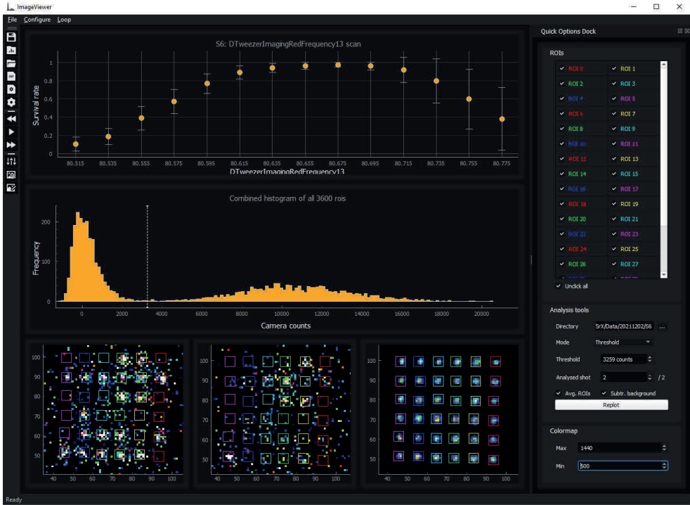
FIGURE 4.3: A screenshot of the GUI of our image viewer software. In the upper left we have a number of buttons for functions. In the center three panels we have the plot of the data set for the selected image number, the histogram of the selected data point and imagenumber, and three tweezer array images. The three images are the last two images taken (of the same experimental run) and an average image for the selected data point and image number. The data set displayed here is one of the data sets from Fig. 2.3. On the right side we have the list of ROIs to be included along with additional quick options for plotting the results.
