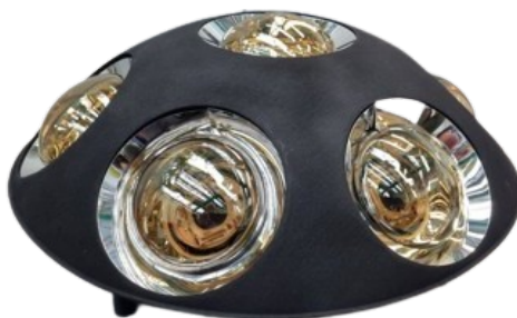
Figure 3. multiPMT holder with reflectors and PMTs installed.
