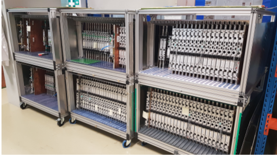
Figure 5.35: Picture of GE1/1 chamber storage in the GEM laboratory at CERN. The GE1/1 chambers are sent from the different production/testing sites to CERN after passing the QC5 gain uniformity test. In total, 161 validated GE1/1 single chambers are stored.
