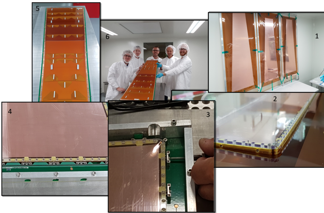
Figure 5.15: Collection of pictures taken at Ghent while assisting the Ghent production team during an assembly of a GE1/1 chamber. Clockwise, one can see highlights of the assembly procedure in chronological order: 1) Three GEM foils as they are received by the production site. The trapezoidal shape of the active foil area can be seen. The protruding part of the polyimide is removed during the assembly. 2) Corner of the trapezoid with the stack of GEM foils. In yellow, the spacers can be seen. 3) Stack of GEM foils put on top of the drift board. By applying a predefined torque to the pullout screws, the GEM foils are stretched. 4) Large base of the trapezoid. The spacers (yellow), brass pullouts, the external gas frame (green) and the o-ring (black) are shown. 5) Fully assembled GE1/1 chamber. The readout board with the 24 sectors can be seen. 6) Ghent and Aachen team after the assembly in the clean room.
