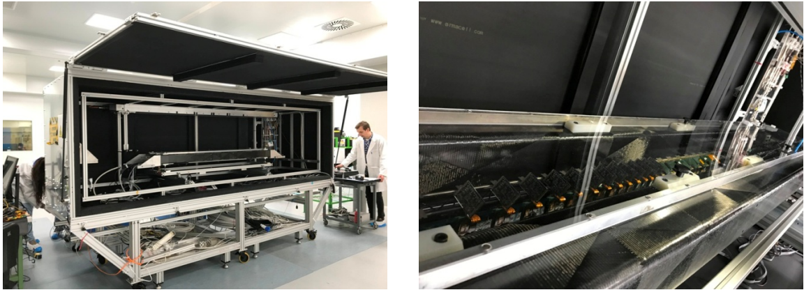
Figure 8.5: Left: The demonstrator testing box with the longeron. In a light tight environmental box the longeron is shielded from external factors and CO 2 cooling and dry air supply allowed controlled environmental conditions. Right: A view on the demonstrator with the inclined modules visible on the left side.
