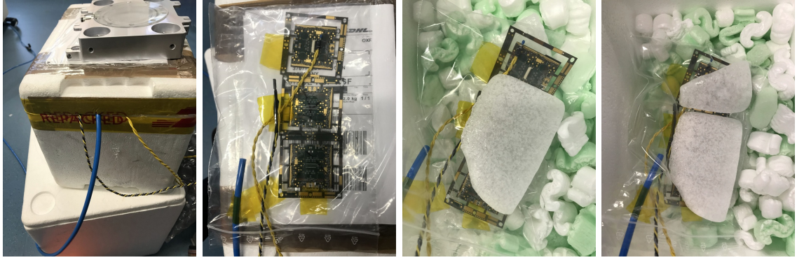
Figure 7.18: Foam box used for the cycling tests with dry ice. The dry air supply and the sensors inside the bag are used to monitor and maintain appropriate environmental conditions.
