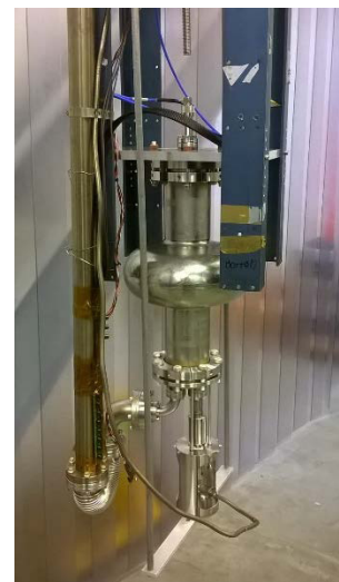
Figure 1: Single-cell cavity N3 attached to a vertical test stand with a variable input coupler.
