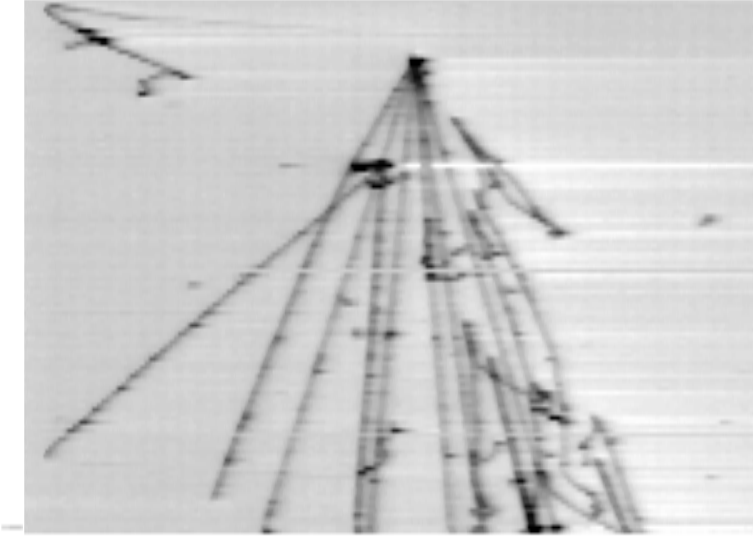
Fig. 22. An example of recorded neutrino interaction in a 50 liter Liquid Argon TPC prototype exposed at the CERN \nu beam. The neutrino comes from the top of the picture. The horizontal axis is the time axis (drift direction) and vertically is the wire number. The visible area corresponds to 47 \times 32 \text{ cm}^2
