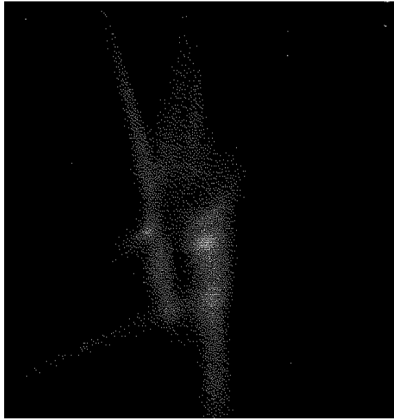
Figure 9.18: Phosphor screen focussed image of dark current from gun
