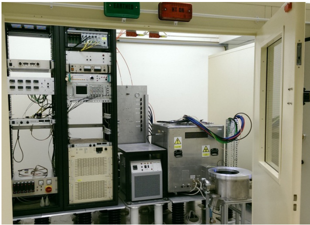
Figure 1: Ion source equipment in the VESPA high voltage enclosure.
