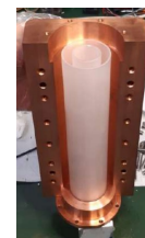
Hybrid dielectric-Nb 3 Sn cavity for INFN QUAX haloscope
