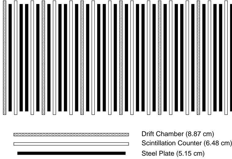
Figure 3.6: Layout of a CCFR target module. A scintillation counter is positioned after every two steel plates and a drift chamber is found after every four.
