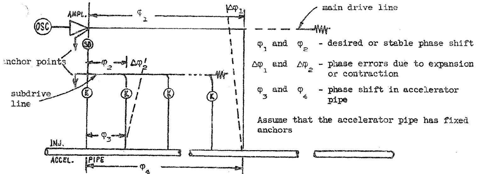
FIG. 1--Schematic drawing of drive system and accelerator pipe showing geometric and rf phase relationship between them.
