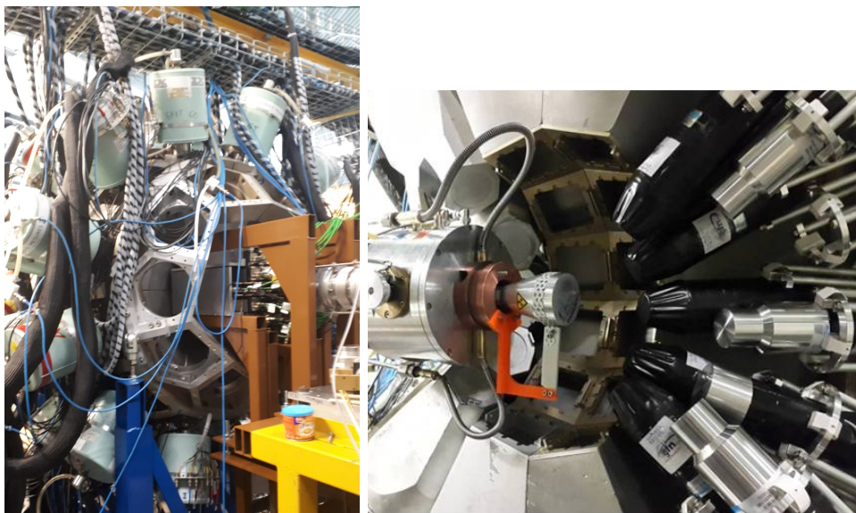
Fig. 2. Left — picture taken of the experimental setup of \nu -ball coupled to the PARIS array. Right — picture of the \nu -ball array coupled to the LICORNE neutron production chamber.
