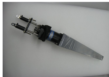
Figure 3. BGO crystal coupled to the photomultiplier.
