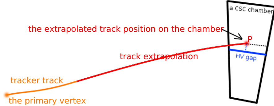
Figure 3.28: Sketch of the track extrapolation on the CSC chamber. The two dotted lines are the required distances from the extrapolated track position to the chamber edge and HV gap.
