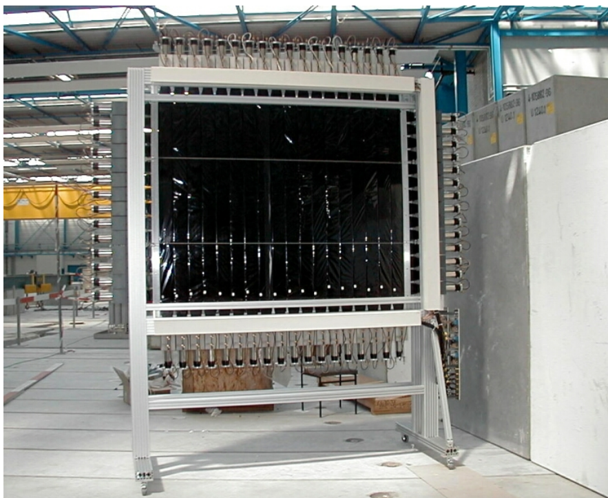
FIGURE 2.11: The heavy fragment branch Time of Flight Wall. Two perpendicular planes of plastic scintillator paddles are used to determine the charge and \beta velocity of the impinging heavy ions.
