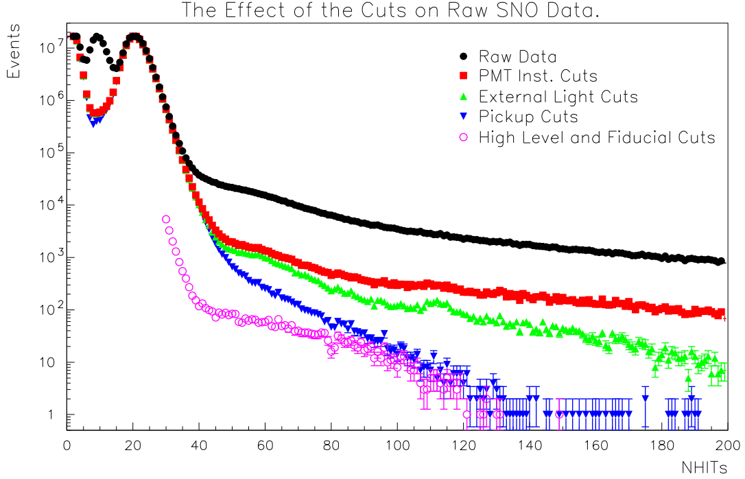
Fig. 7.1: N_{\text{Hit}} distribution for the raw data and data with DAMN, \theta_{ij} and ITR cuts applied. Figure taken from [75].
