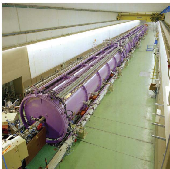
Figure 1: Top: Overview of the existing UNILAC. Left: View into the UNILAC tunnel along the 55 metres long post-stripper. Right: View into the Alvarez DTL cavity during maintenance.
