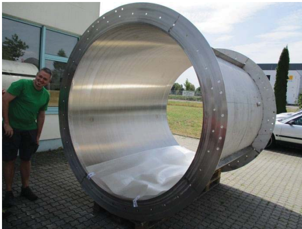
Figure 10: Dummy cavity (L=2.5m, D out =2.4m) at the factory acceptance test (FAT).
