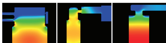
Figure 4: Simulated log-scale electric field distribution (ACE3P) for ASC (left), GW (center), and MC (right) with emphasis on the coupler region.
