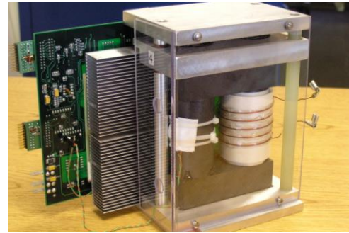
Figure 4: H-bridge driver and transformer module assembly.
