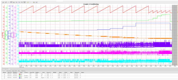
Figure 2: Coupler conditioning overview from top to bottom: magnitude of the forward power (red), duty cycle (green), RF pulse width (blue), vacuum (orange), arc detection (vacuum in magenta and air side in violet) and electron pick-up signals (cyan).
