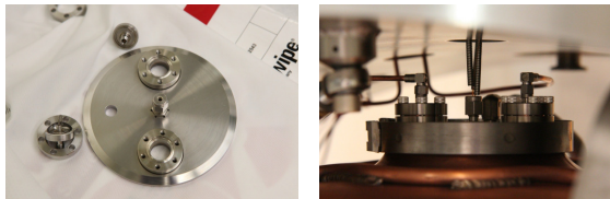
Figure 2: RF pickup probes installed through the top hat of the cavity. SMA connectors are used.
