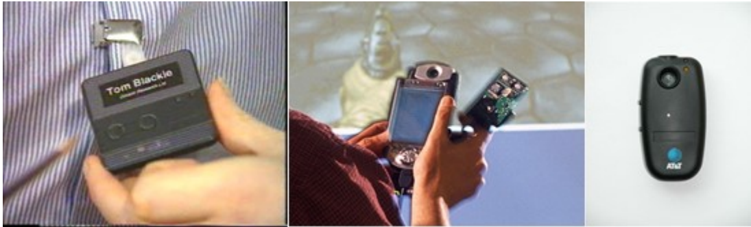
Figure 16 - Photos of dedicated infrastructure high resolution positioning systems (a) Active badge, (b) Cricket, (c) Bat
