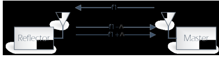
Figure 56 - Signals transmitted between Master and Reflector units The master generates a wave of frequency f_1 , which is “reflected” in frequencies f_1 - \Delta f and f_1 + \Delta f .
